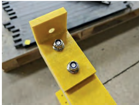
Fig. 3.3: Assembly of floor brackets
